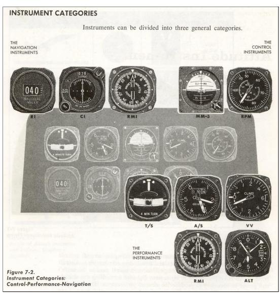
Figure 26. Flight instrument categories (US Air Force Manual 51-38, 1954).
