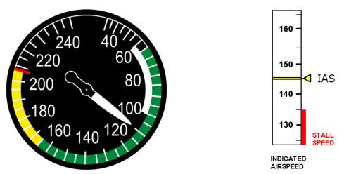
Figure 12. Conventional airspeed indicator (Wikipedia 2014). Figure 13. State of the art airspeed indicator (Wikipedia 2014).
