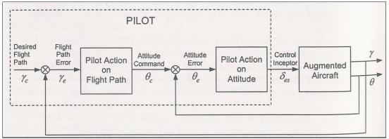
Figure 25. The series pilot model<sup>22</sup>
