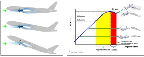
Figure 5. Aerodynamic Stall (D. Carbaugh, Boeing 2010).
