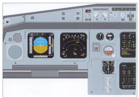
Figure 11. Airbus standard flight display layout (Airbus).
