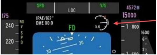
Figure 8. Boeing AOA indicator (Boeing 2013).
