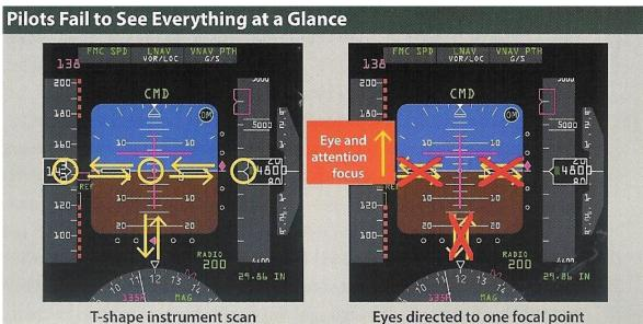
Figure 28. T-shape instrument scan (Boeing 2014).
