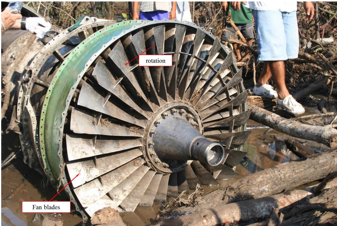
Figure 12: No. 1 engine fan stage as observed at the accident site
