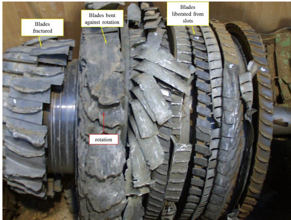
Figure 7: Historical example of blade damage that occurs at impact with the rotor at a high rotational speed
