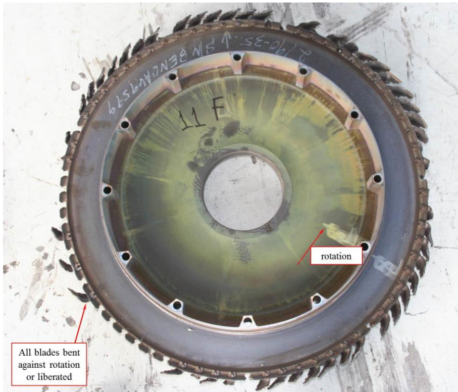
Figure 10: Typical compressor rotor from the No. 2 engine
