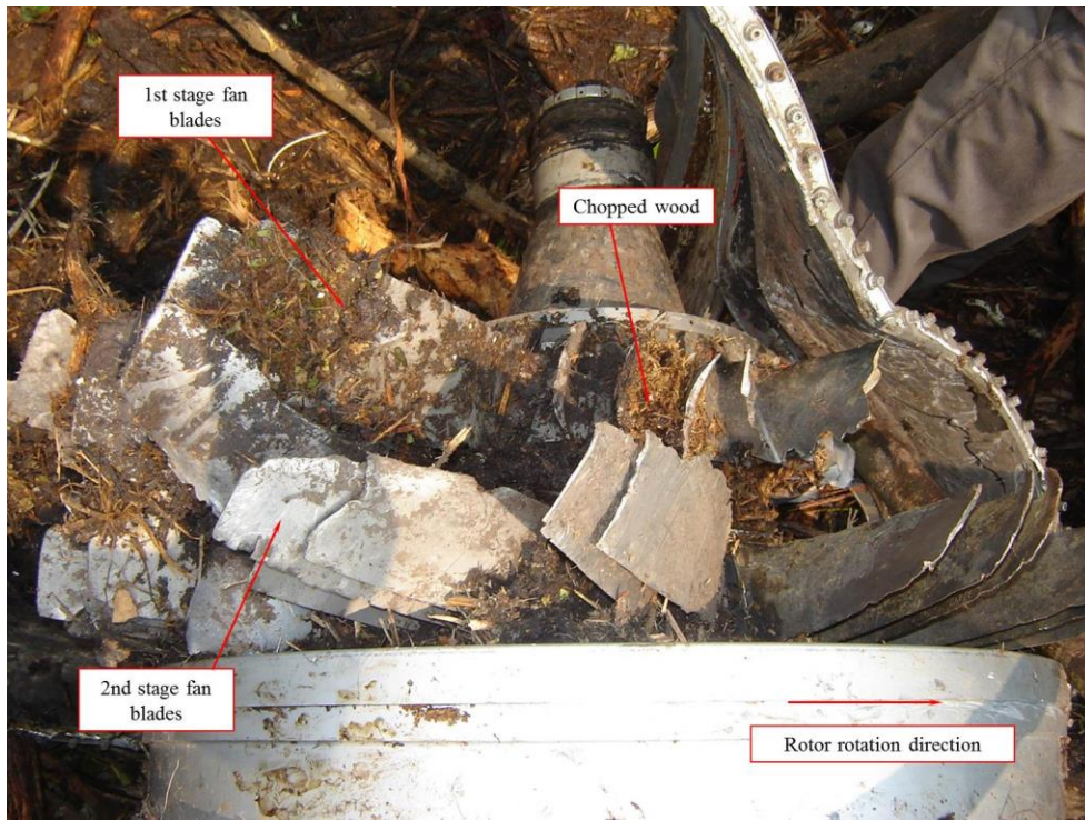
Figure 9: Representative fan stage damage for the No. 2 engine (Photo Credit: CIAA Peru)
