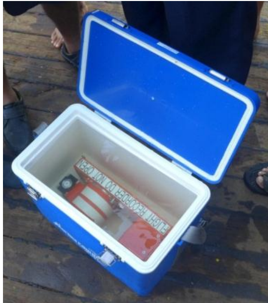
Figure 11: CVR placed in a water filled cooler box
