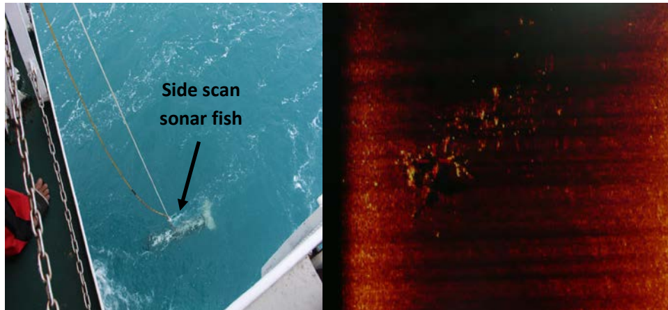
Figure 5 (Left): Side scan sonar fish being lowered into the water (Right): Possible debris field identified by MPA's side scan sonar
