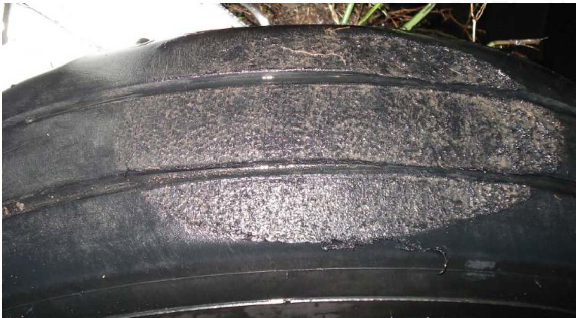
Figure 16 – Reverted rubber evidence on the tire surface (ref. 6)
