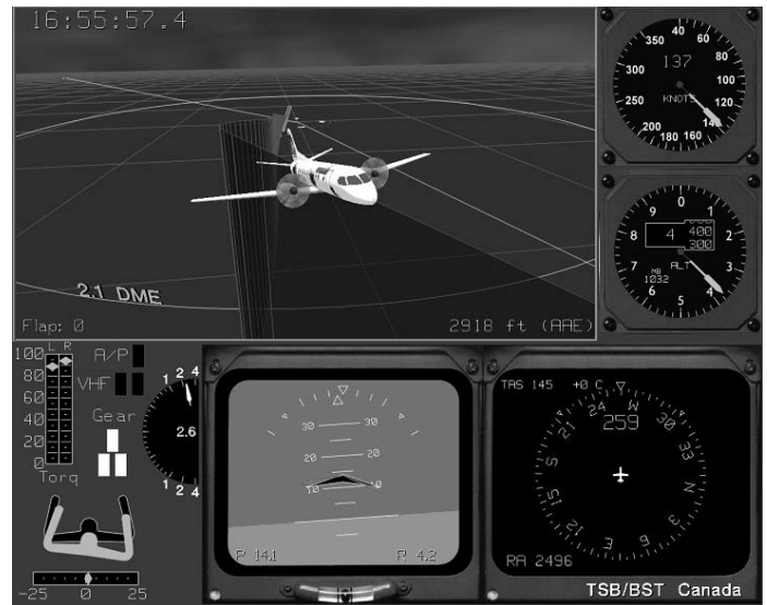
Figure 2 (above). Flight animation developed by the TSB to support the investigation team (courtesy the TSB). Figure 3 (left). Planned route, instructed route, and flight path to crash site.
