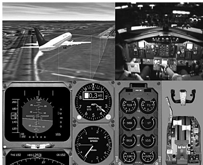
Figure 5: Simulator session animation replay using the same core technology as the accident investigation replay (courtesy Oxford Aviation).
