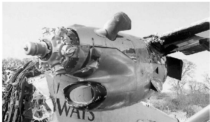
Figure 6: Left engine nacelle with external intake and one exhaust stack visible after wreckage recovery.
