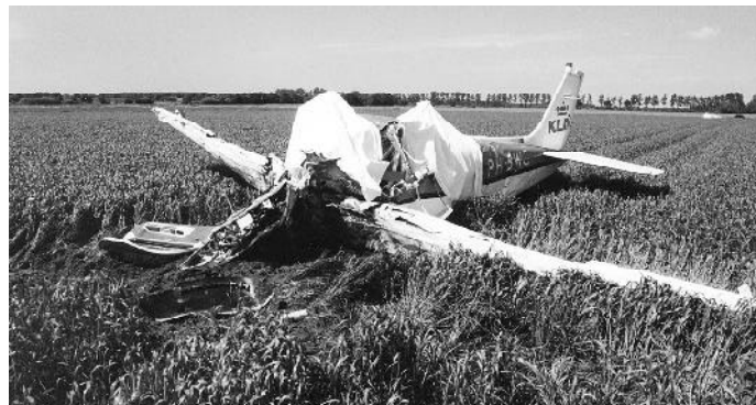
Beech Bonanza PG BWC aircraft 1. The main wreckage vertically impacted the ground.
