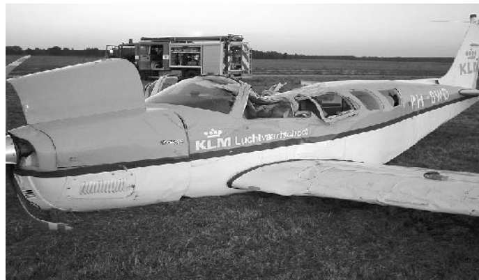
Aircraft 2 was found in a meadow. From the track in the meadow, it could be determined that a rather smooth gear-up landing was executed. The cockpit roof was heavily damaged and scratched, and the left upper wing was dented.
