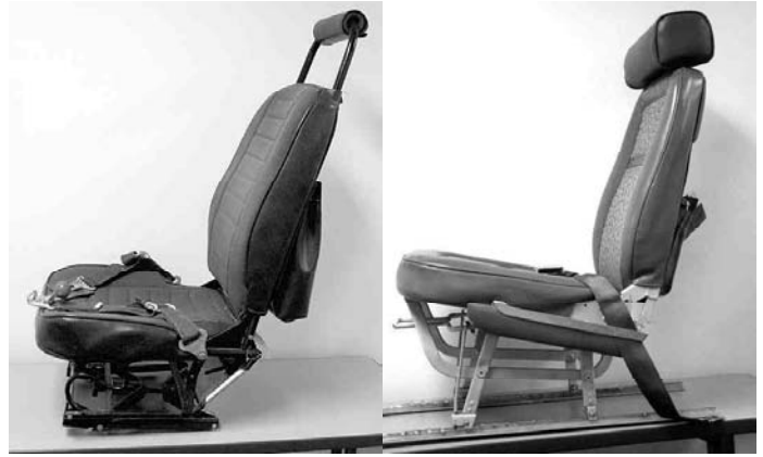
Left, S-tube seat. Right, pre-1988 general aviation seat.
