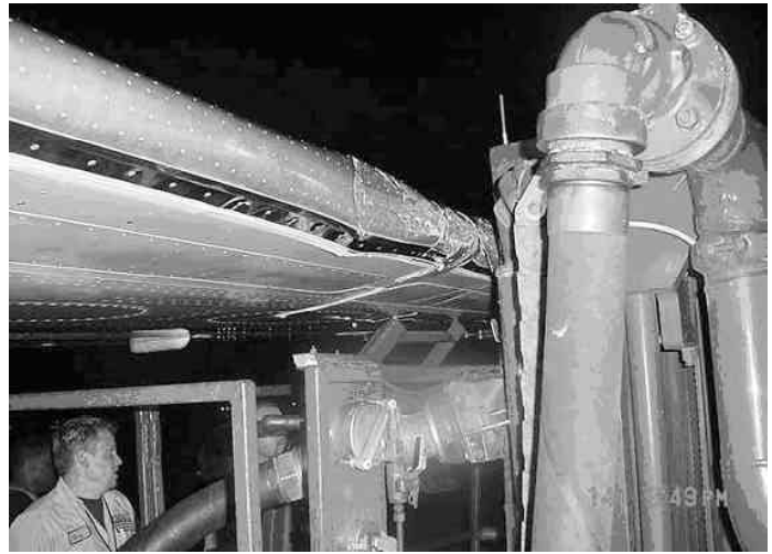
Figure 1: Leading edge slats 4 and 5 damaged.
