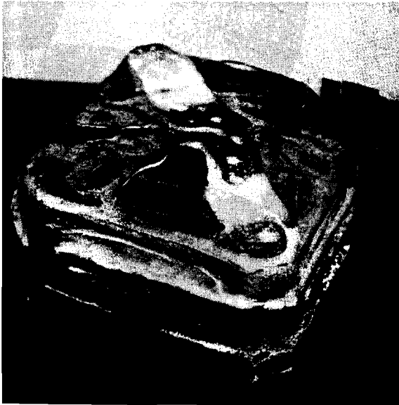
FIG. 3: INSULATION PACKAGE OF HEAT-DAMAGED COCKPIT VOICE RECORDER
