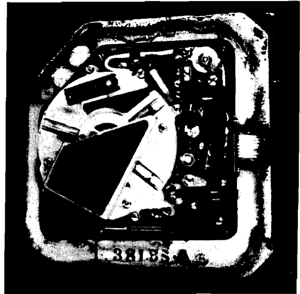
FIG. 4: TAPE TRANSPORT OF HEAT-DAMAGED COCKPIT VOICE RECORDER
