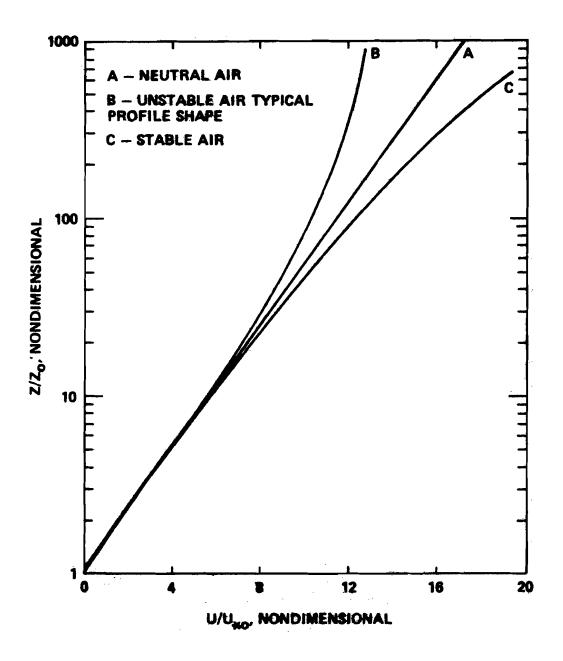
FIGURE 1. WIND PROFILES FOR VARIOUS STABILITY CONDITIONS OVER HORIZONTALLY HOMOGENEOUS TERRAIN. u, AND DENOTE THE SURFACE FRICTION VELOCITY AND ROUGHNESS.
