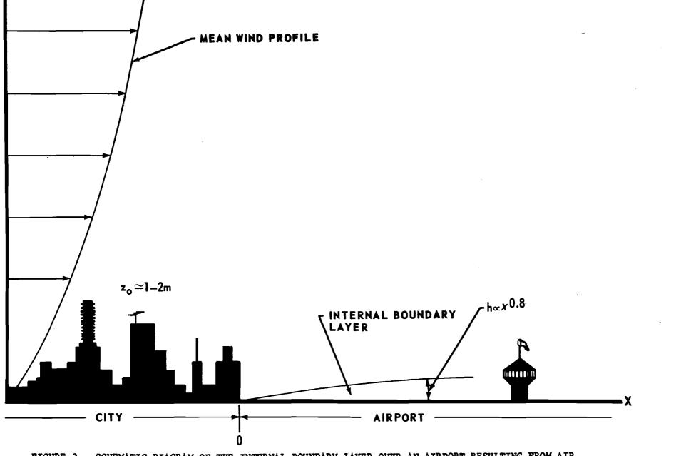
FIGURE 3. SCHEMATIC DIAGRAM OF THE INTERNAL BOUNDARY LAYER OVER AN AIRPORT RESULTING FROM AIR MOVING FROM ROUGH TO SMOOTH TERRAIN.
