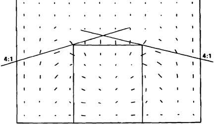
PLANE VIEW OF THE VELOCITY FIELD THAT EXISTS DIRECTLY BEHIND THE STRUCTURE AS SEEN FROM DOWNSTREAM
