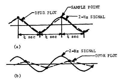
FIGURE D-3. 2-Hz acceleration signal with a 4-Hz sampling frequency assuming peaks of signal (a) coincide with sample times, and (b) do not coincide with sample times.
