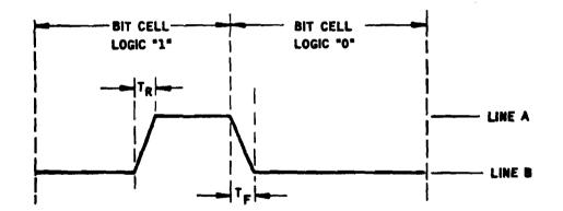
WAVEFORM CHARACTERISTICS (PER ARING 573) HARVARD BI PHASE CODE (DFDR INPUT SIGNAL)
