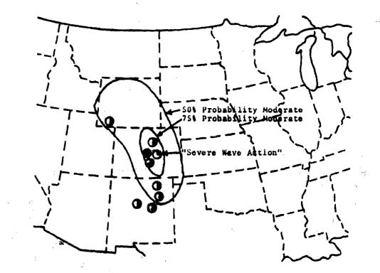
Figure 4. Forecast zone of mountain wave turbulence is shown with two degrees of probability in this figure. Verification is illustrated by later actual encounters of moderate to severe CAT occurring during the valid forecast period of 6 hours. Forecast also called for turbulence to be expected between Flight Levels 250 and 400. Symbols for turbulence intensity are shown in Figure 5.
