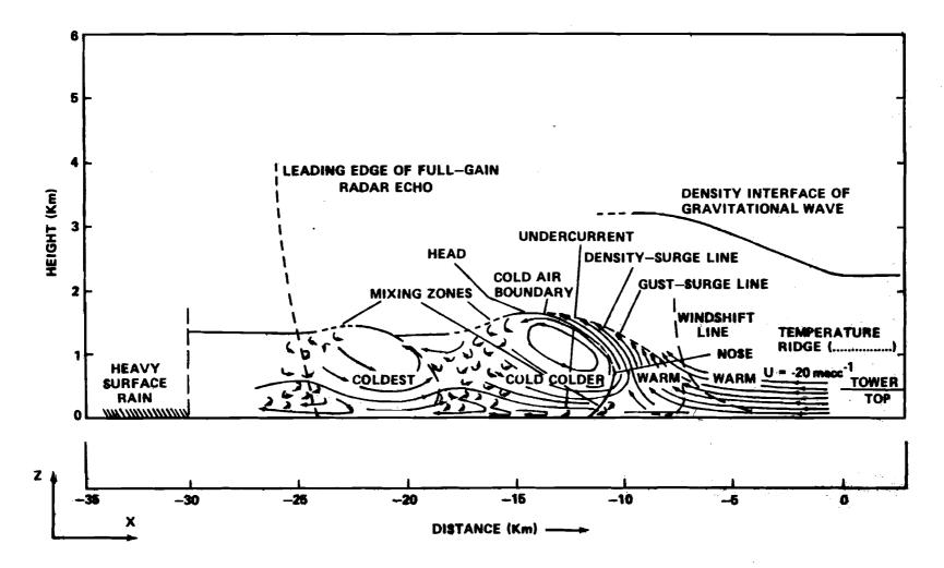
FIGURE 5. SCHEMATIC DIAGRAM OF THE STRUCTURE OF THE COLD AIR OUTFLOW FROM THUNDERSTORMS [58, 59].
