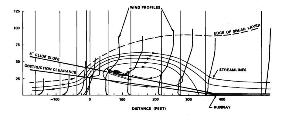
FIGURE 8. FLOW OVER A FENCE AND THE TAKE-OFF FLIGHT PATH OF A STOL VEHICLE THROUGH THE ASSOCIATED FLOW DISTURBANCE.
