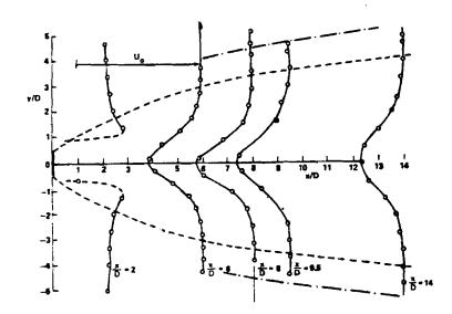
FIGURE 22. VELOCITY PROFILES IN THE WAKE OF A TWO-DIMENSIONAL FLAT PLATE -- TOTAL HEAD WAKE BOUNDARY -- TURBULENCE-FREE WAKE BOUNDARY [31].
