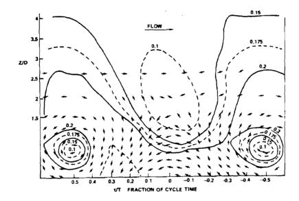
FIGURE 23. CONDITIONALLY AVERAGED CYCLE OF UPPER HALF OF FLAT PLATE WAKE AT x/D = 6, VORTICES STATIONARY. CONTOURS JOIN POINTS OF EQUAL FLOW SPEED,  $\rightarrow$  LOCAL FLOW DIRECTION.
