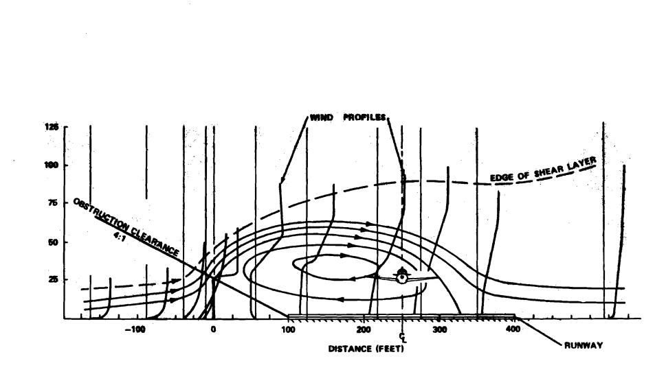
FIGURE 9. FLOW OVER A FENCE AS IN FIGURES 6 AND 8 FOR THE CROSSWIND CASE.
