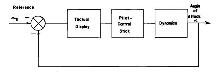
Fig. 1. Control Loop for Angle of Attack
