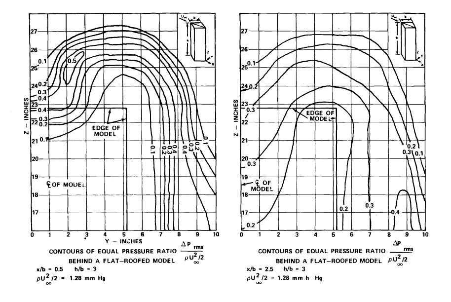
FIGURE 19 (continued). STRUCTURE OF LONGITUDINAL BUILDING VORTICES [42].
