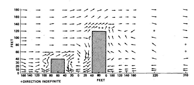
FIGURE 15. SLAB AND LOW BUILDING IN A GRADIENT WIND VELOCITY.
