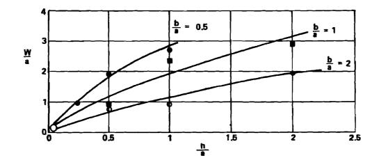
FIGURE 14. WAKE GEOMETRIES BEHIND A THREE-DIMENSIONAL BLUFF BODY [43].
