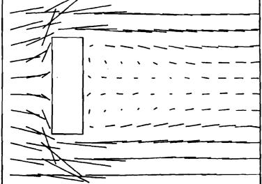
PLANE VIEW OF THE VELOCITY VECTORS AS SEEN FROM ABOVE A SIMULATED BUILDING.
