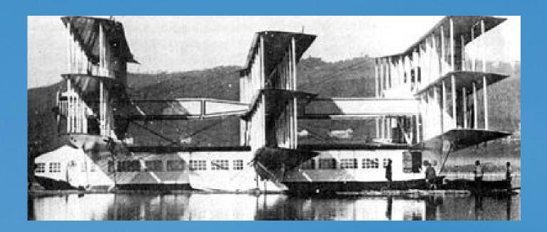
The *Caproni Ca 60 Noviplano*, dubbed the 'Capronissimo', was an absurd aircraft which featured three sets of triplane wings set above a giant fuselage which resembled some sort of luxury houseboat.
