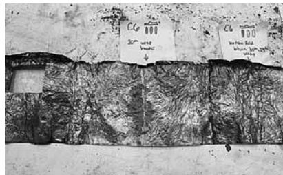
Figure 13: Cell 6 electrode with anomalous areas of interest.
