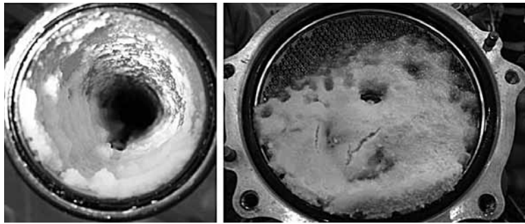
LEFT—Figure 1: Fuel tube and FOHE ice.
