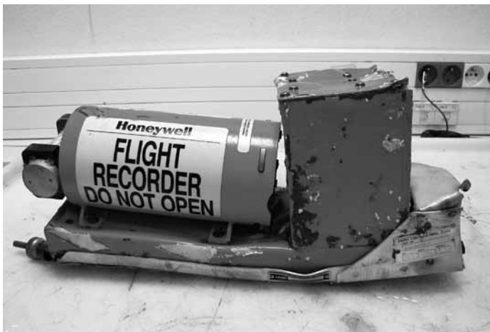
FDR—recovered and ready for inspection.
