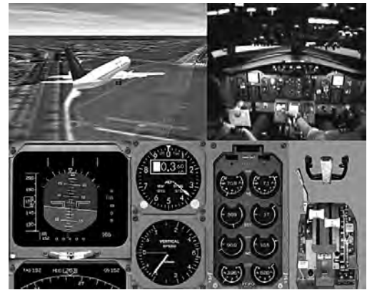
Figure 5: Simulator session animation replay using the same core technology as the accident investigation replay (courtesy Oxford Aviation).
