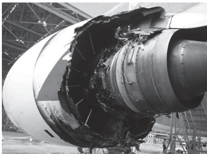
Figure 6. Uncontained engine disc failure, A380 (2010)
