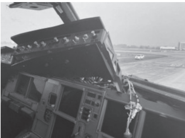
Figure 8. Loss of right-hand windshield in flight, A319 (2018)
