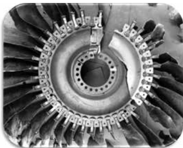
Recovered fragments of the Stage 1 Fan Disk from UA232
