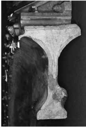
Failure Surface of the Stage 1 Fan Disk from UA232
