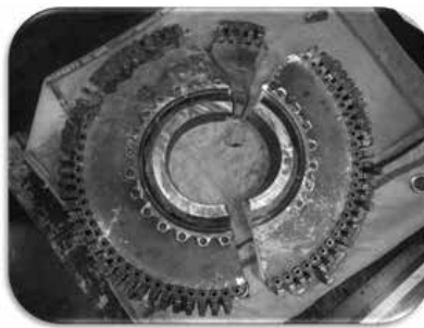
Recovered fragments of the High Pressure Turbine Stage 2 Disk from AA383
