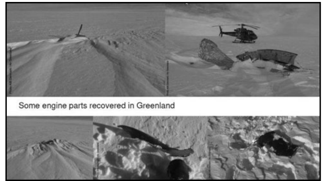
Figure 10. The BEA and AIB of Denmark use helicopters to locate and recover the larger, aerodynamic engine components.
