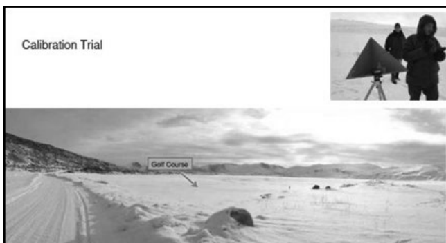
Figure 6. A calibration test piece is mounted on a tripod and positioned on a snow-covered golf course with its exact angle and GPS position noted.
