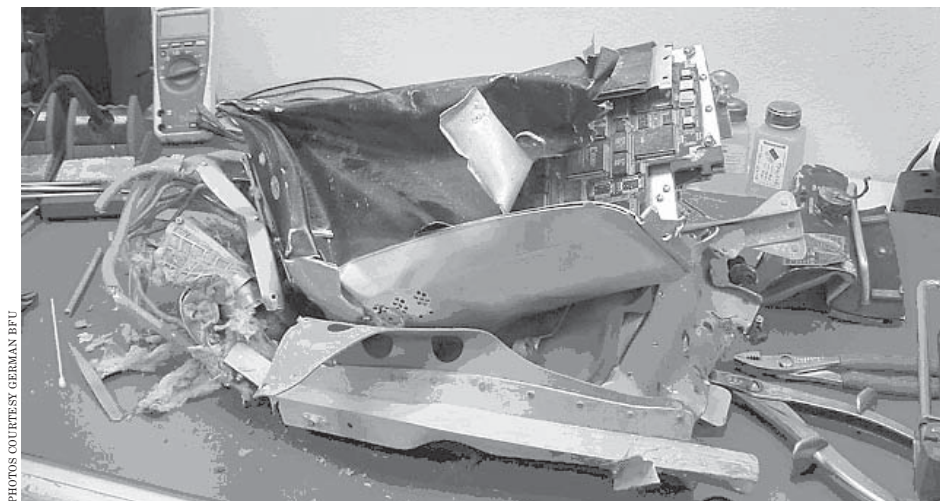
The damaged ACAS/TCAS computer of the TU 154M.
