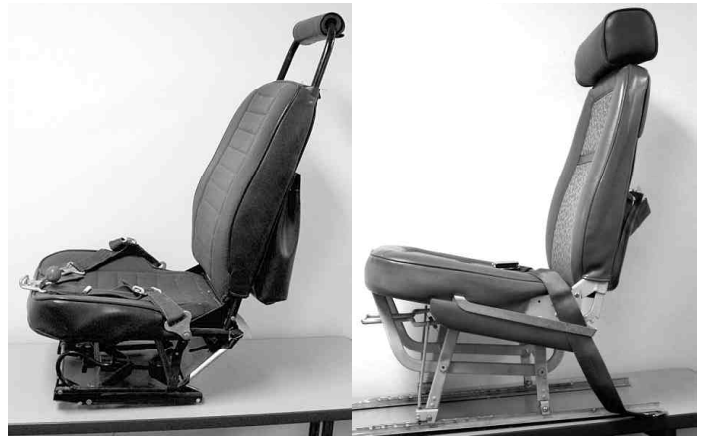
Left, S-tube seat. Right, pre-1988 general aviation seat.
