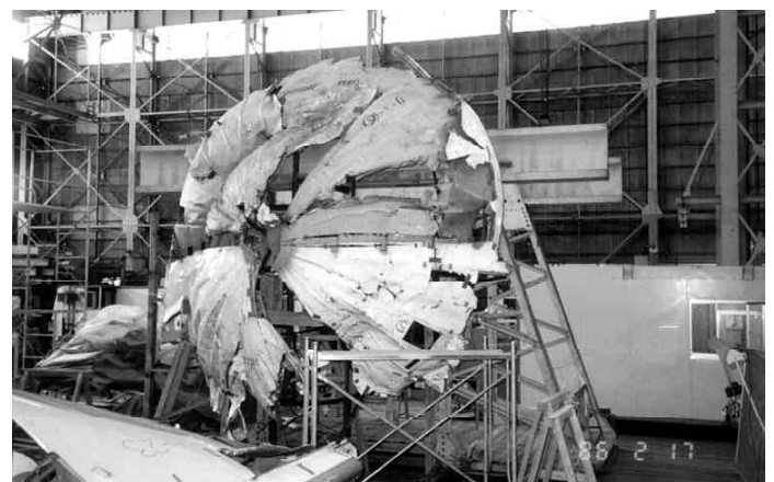
Aft pressure bulkhead 3-D mockup (JAL B-747, 1985).
