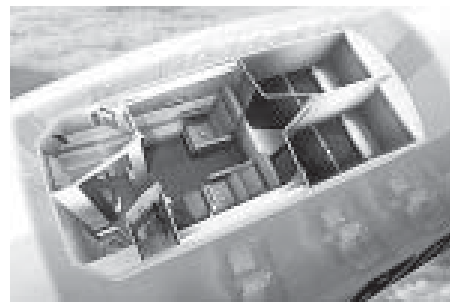
ABOVE: Overhead crew rest—Putting the crew rest area in the crown of the airplane frees up space for more revenue-generating seats. BELOW: The Boeing 777 has the spacious cross-section required to incorporate roomy berths and business-class-comfort seats into overhead rest quarters.
