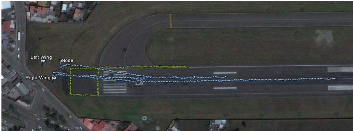
Figure 2 - Recorded GPS tracking along the runway threshold used as reference for calibration
