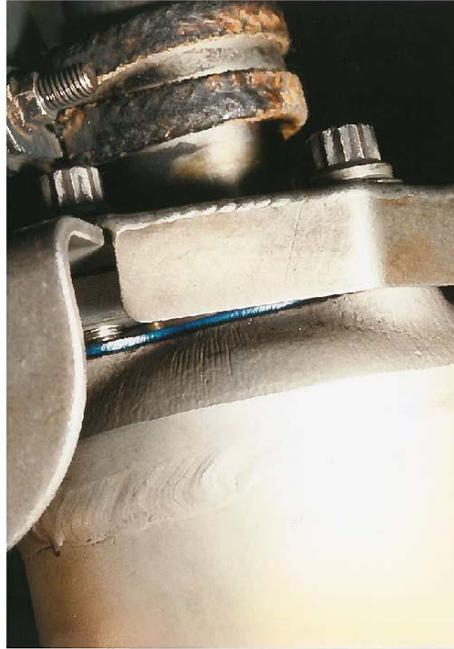
Figure 5: CF6 Gap at Leaking Flange
