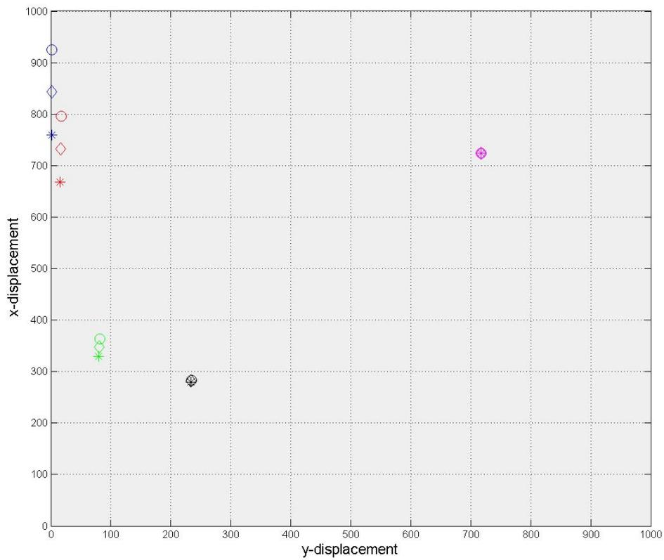
Figure 4 - The effect on final wreckage location of changing initial forward velocity for a simulated small aircraft accident.  $C_B=10,000$ ;  $C_B=1,000$ ;  $C_B=100$ ;  $C_B=10$ ;  $C_B=1$ .
