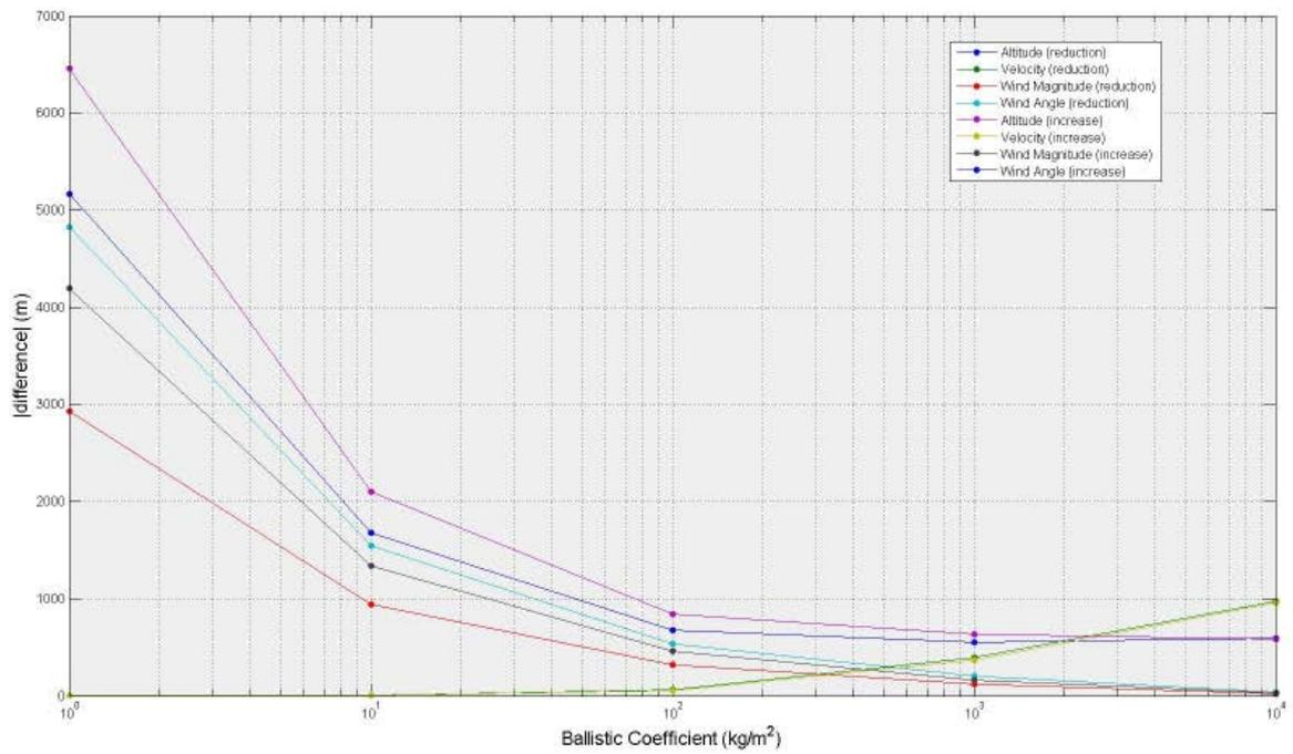
Figure 5 - Variation in magnitude of distance from position in reference case for of various parameters and  $C_B$
