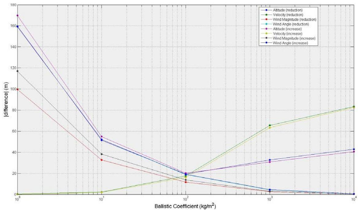
Figure X6 - Variation in magnitude of distance from position in reference case for combined of various parameters and  $C_B$
