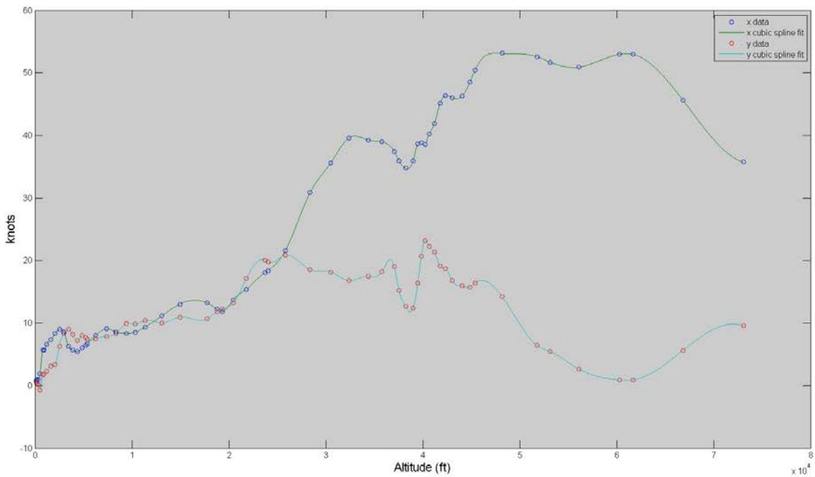
Figure 2 - Cubic spline fit for x and y components of wind data
