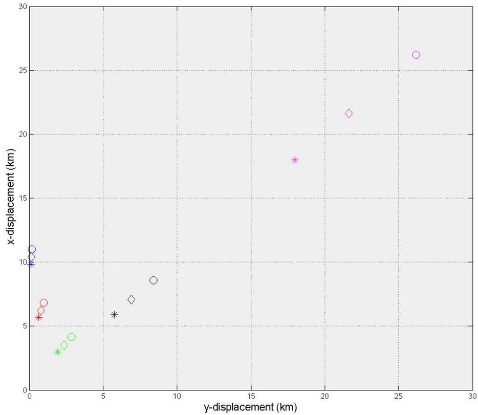
Figure 3 - The effect on final wreckage location of changing breakup altitude for a simulated large aircraft accident.  $C_B=10,000$ ;  $C_B=1,000$ ;  $C_B=100$ ;  $C_B=10$ ;  $C_B=1$ .
