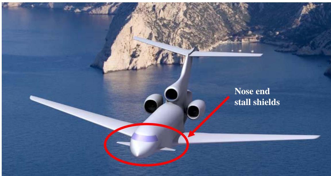
Fig 2. Stall shields at the nose end of a T-tailed aircraft
