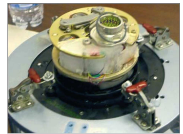
Amount of ice in the housing of the Angle of Attack sensor after the water exposure test
