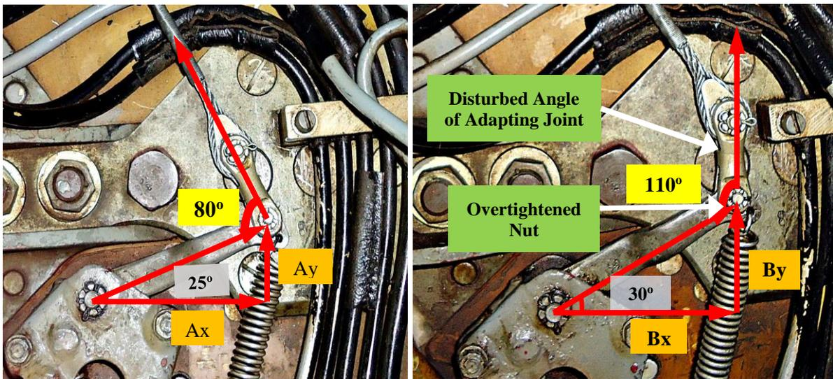
Figure 1. Change of Adapting Joint angle. The left figure shows the normal/desired angle of  $80^\circ$ , whereas the figure on right shows the disturbed angle of  $110^\circ$  due to overtightened nut.
