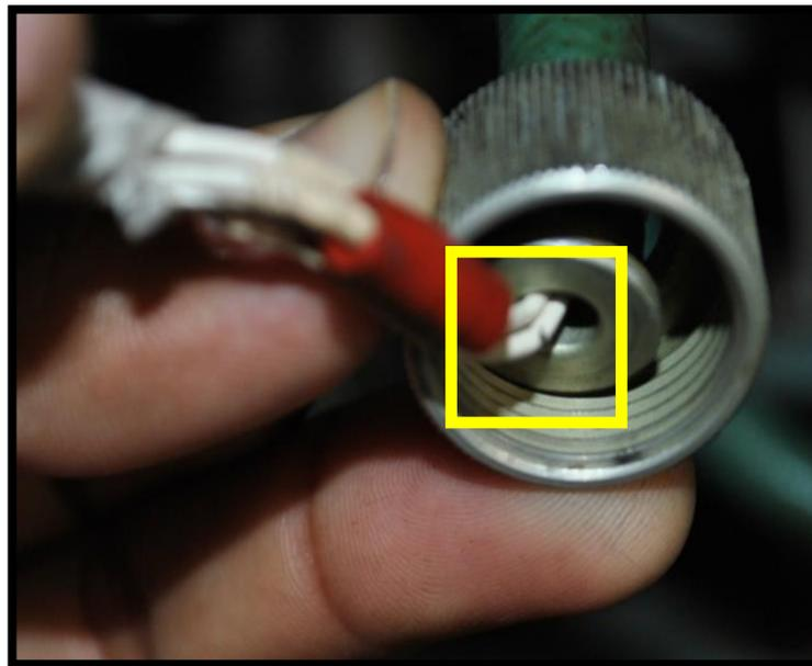
*Figure 2. Hairline crack on electrical wire due to chaffing.*
