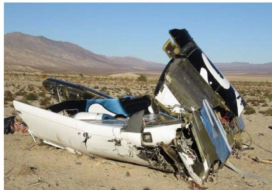
Figure 5: SpaceShipTwo Wreckage
