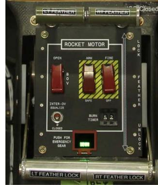
Figure 4: Feather Lock Handle – Unlocked Position
