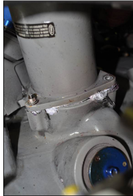
Figure 8. Cougar 91 missing filter bowl stud
