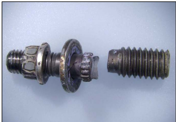
Figure 6. S-92A broken MGB filter bowl mounting stud
