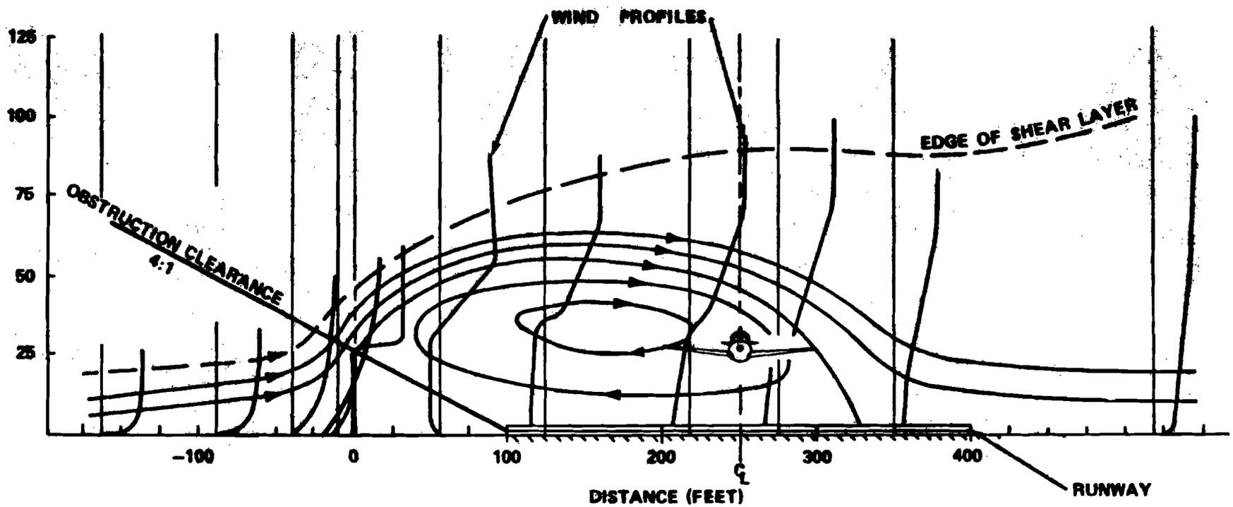
FIGURE 9. FLOW OVER A FENCE AS IN FIGURES 6 AND 8 FOR THE CROSSWIND CASE.
