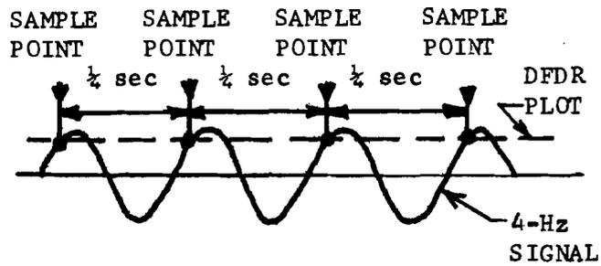
FIGURE D-1. 4-Hz acceleration signal with a 4-Hz sampling frequency.
