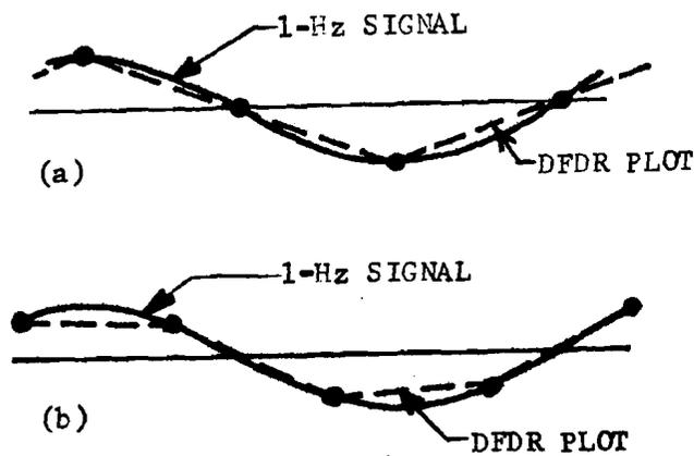
FIGURE D-4. 1-Hz acceleration signal assuming (a) coincidence of peaks and sample times, and (b) no coincidence.
