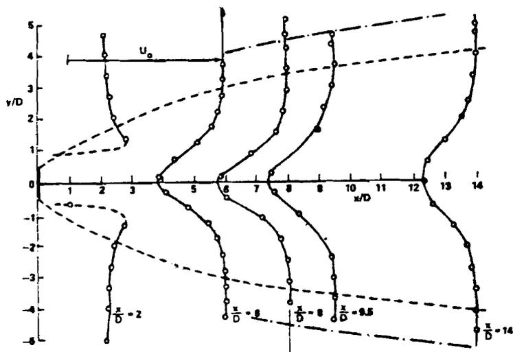
FIGURE 22. VELOCITY PROFILES IN THE WAKE OF A TWO-DIMENSIONAL FLAT PLATE -- TOTAL HEAD WAKE BOUNDARY -- TURBULENCE-FREE WAKE BOUNDARY [31].
