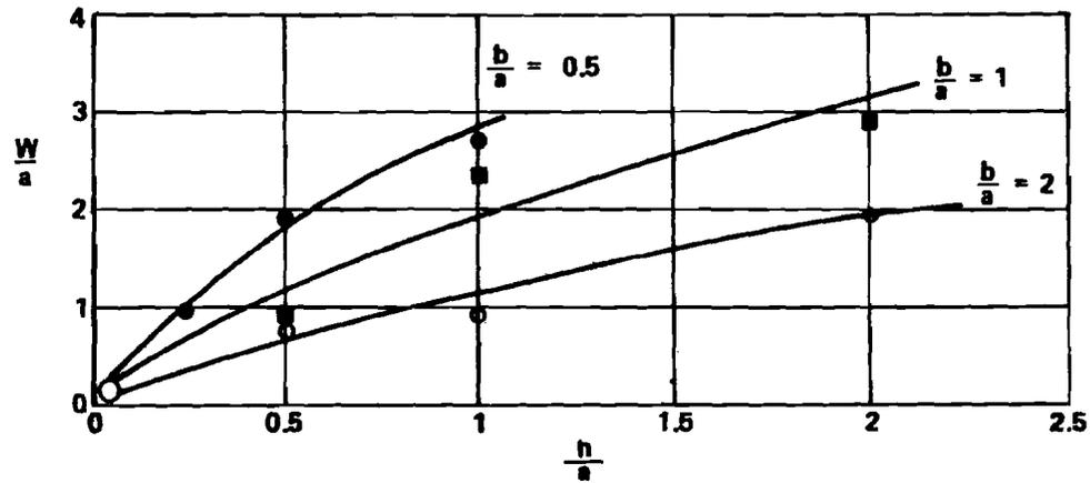
FIGURE 14. WAKE GEOMETRIES BEHIND A THREE-DIMENSIONAL BLUFF BODY [43].
