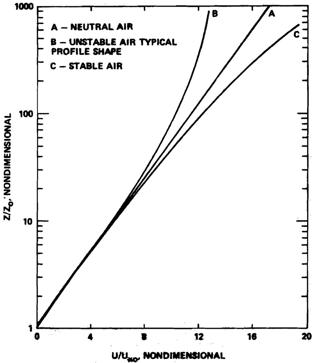
FIGURE 1. WIND PROFILES FOR VARIOUS STABILITY CONDITIONS OVER HORIZONTALLY HOMOGENEOUS TERRAIN.  $u_{*0}$  AND  $z_0$  DENOTE THE SURFACE FRICTION VELOCITY AND ROUGHNESS.
