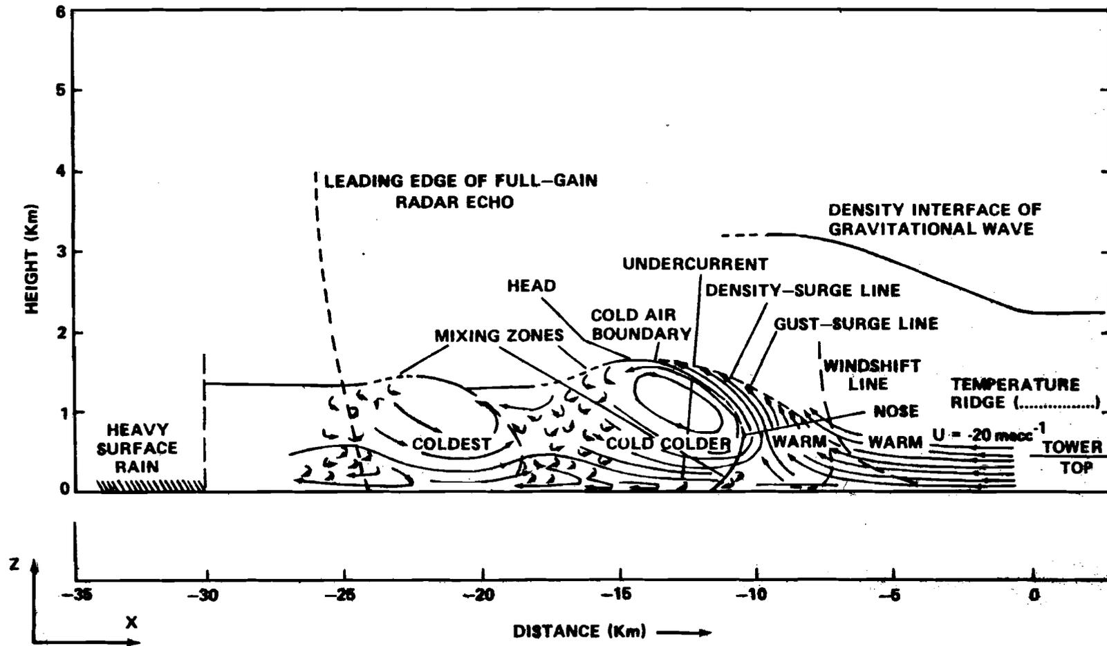
FIGURE 5. SCHEMATIC DIAGRAM OF THE STRUCTURE OF THE COLD AIR OUTFLOW FROM THUNDERSTORMS [58, 59].
