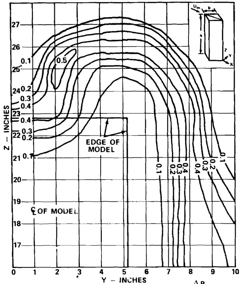
CONTOURS OF EQUAL PRESSURE RATIO  $\frac{\Delta P_{rms}}{\rho U_{\infty}^2 / 2}$
