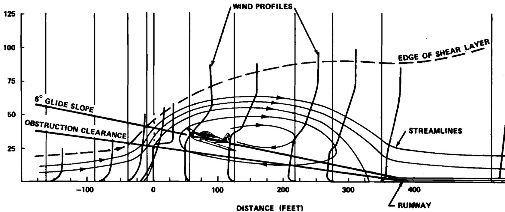
FIGURE 8. FLOW OVER A FENCE AND THE TAKE-OFF FLIGHT PATH OF A STOL VEHICLE THROUGH THE ASSOCIATED FLOW DISTURBANCE.
