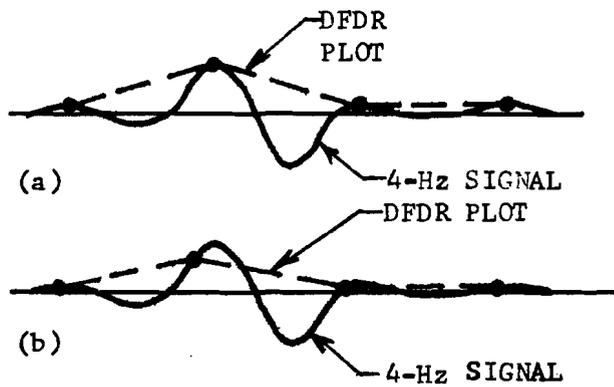
FIGURE D-2. A single cycle of high-amplitude 4-Hz acceleration signal with a 4-Hz sampling frequency assuming peaks of signal (a) coincide with sample times, and (b) do not coincide with sample times.
