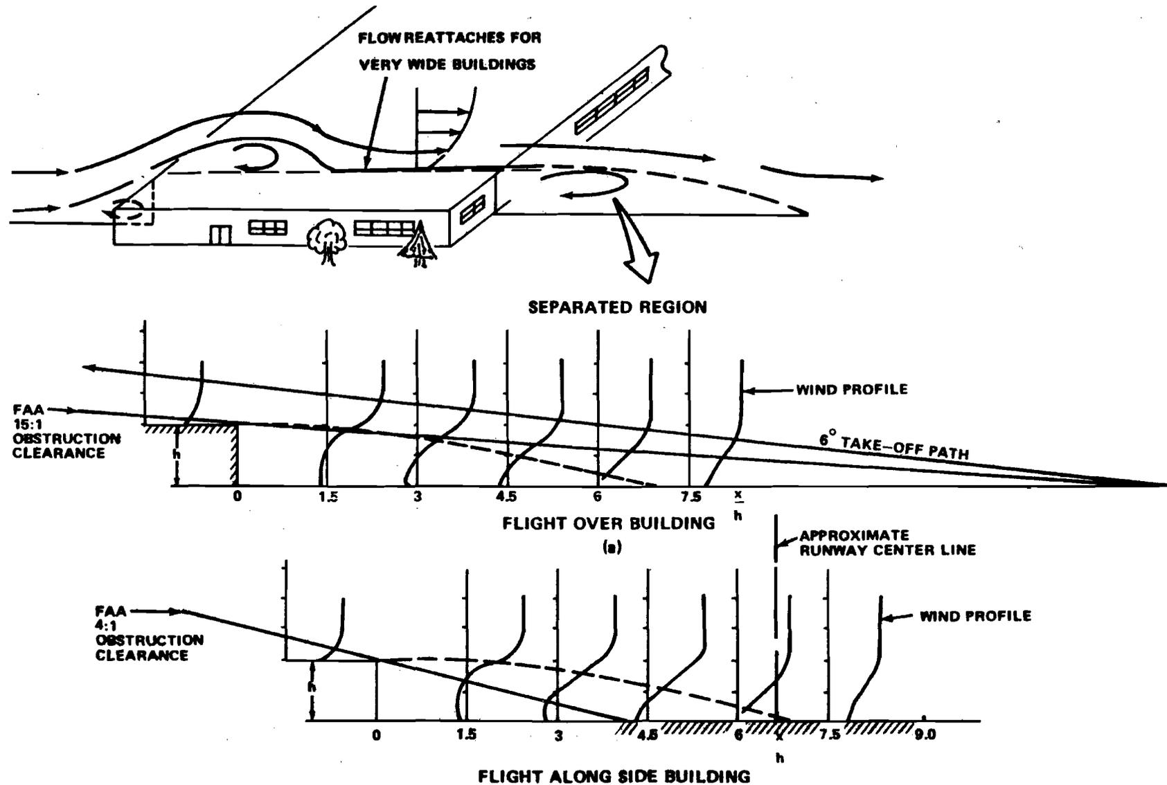
FIGURE 10. FLOW OVER A RELATIVELY WIDE, LOW BUILDING AND RELATIONSHIP BETWEEN THE WIND PROFILES AND THE RUNWAY ORIENTATION RELATIVE TO THE FLOW FOR THE HEADWIND CASE (a) AND THE CROSSWIND CASE (b).
