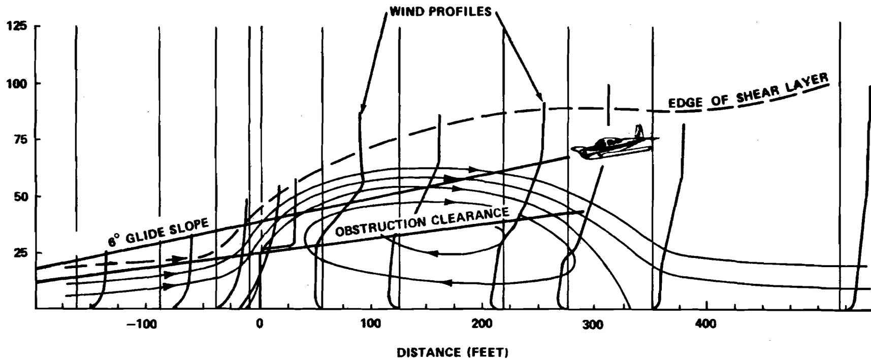
FIGURE 6. FLOW OVER A FENCE AND THE LANDING FLIGHT PATH OF A STOL VEHICLE THROUGH THE ASSOCIATED FLOW DISTURBANCE.
