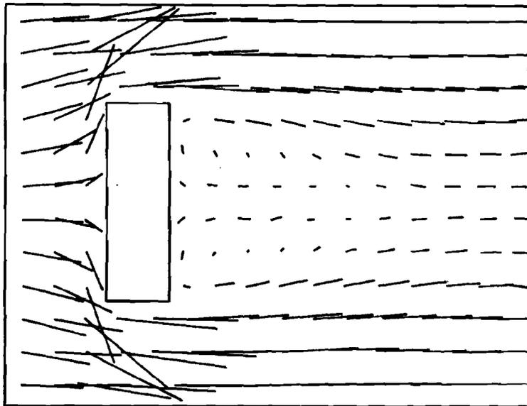
PLANE VIEW OF THE VELOCITY VECTORS AS SEEN FROM ABOVE A SIMULATED BUILDING.
