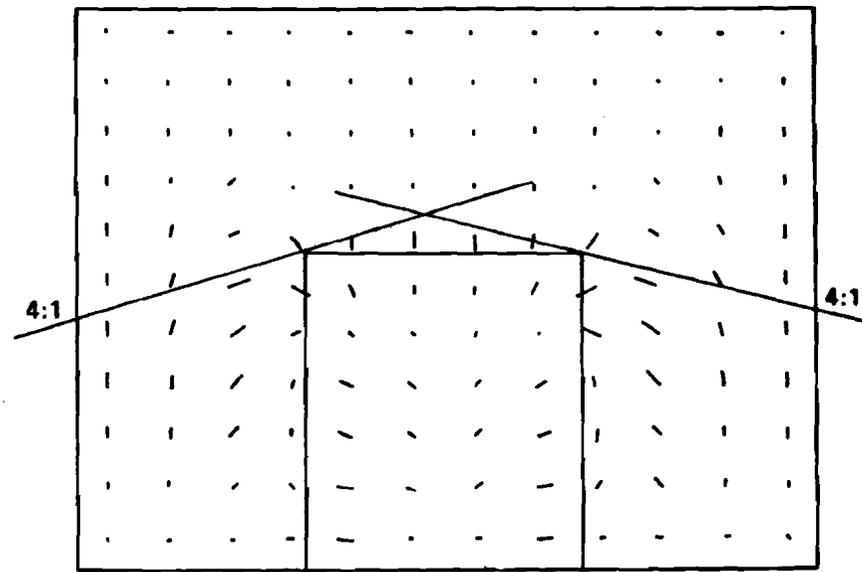
PLANE VIEW OF THE VELOCITY FIELD THAT EXISTS DIRECTLY BEHIND THE STRUCTURE AS SEEN FROM DOWNSTREAM
