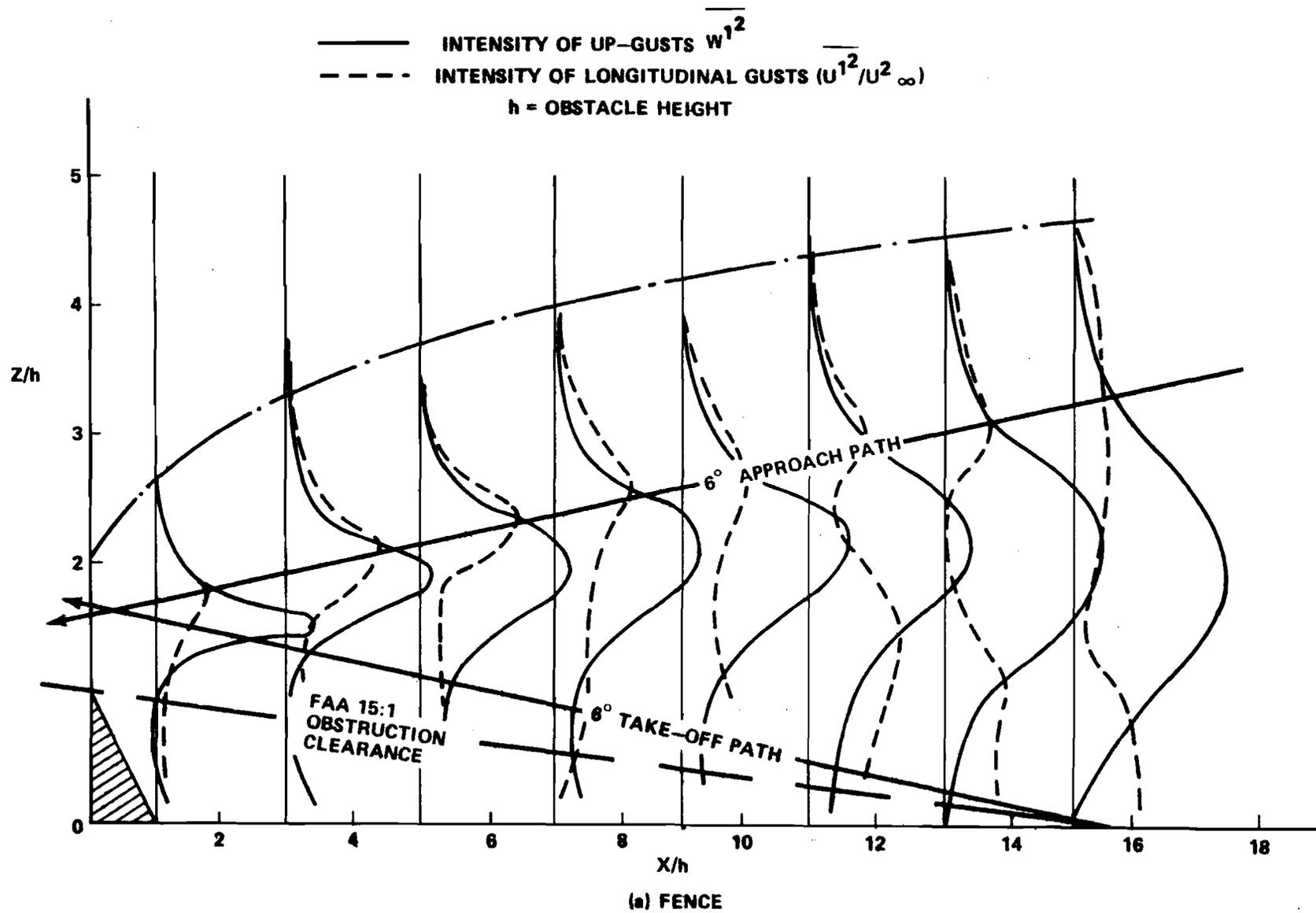
FIGURE 12.a. GUST INTENSITY AS A FUNCTION OF POSITION DOWNSTREAM OF A FENCE AND THE TAKE-OFF AND LANDING FLIGHT PATHS OF A STOL VEHICLE THROUGH THE GUST INTENSITY PATTERN.
