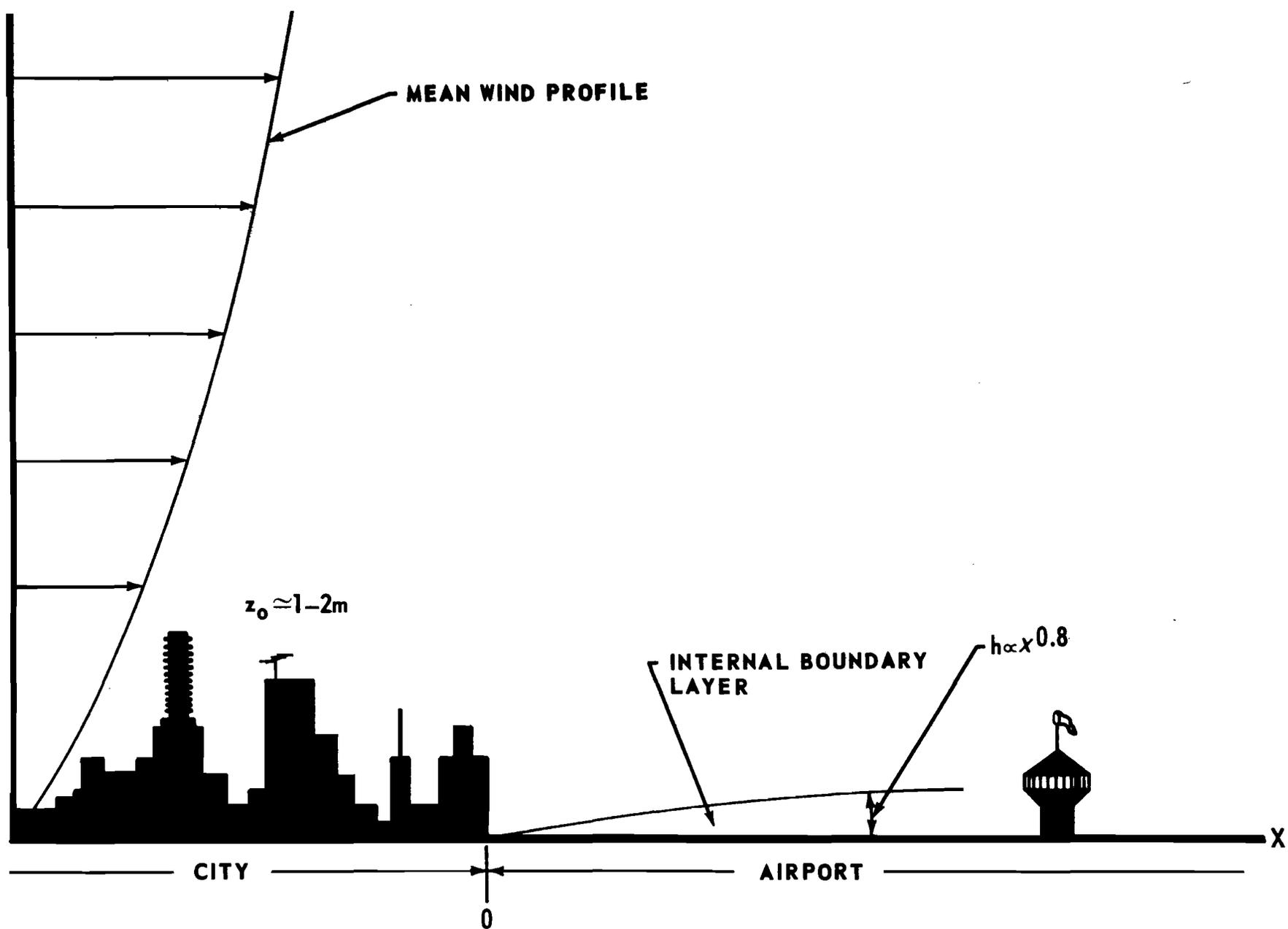
FIGURE 3. SCHEMATIC DIAGRAM OF THE INTERNAL BOUNDARY LAYER OVER AN AIRPORT RESULTING FROM AIR MOVING FROM ROUGH TO SMOOTH TERRAIN.
