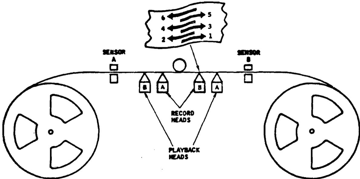
FIGURE 1. Tape motion during recording for LAS DFDR.
