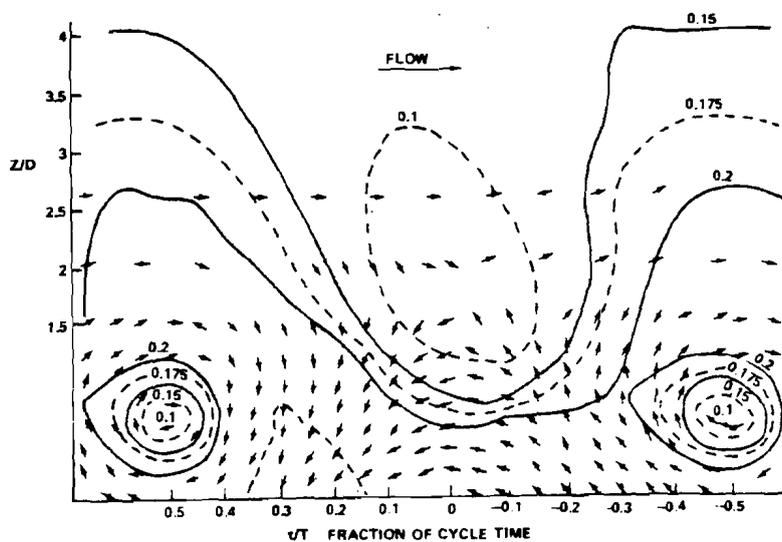
FIGURE 23. CONDITIONALLY AVERAGED CYCLE OF UPPER HALF OF FLAT PLATE WAKE AT  $x/D = 6$ , VORTICES STATIONARY. CONTOURS JOIN POINTS OF EQUAL FLOW SPEED,  $\rightarrow$  LOCAL FLOW DIRECTION.
