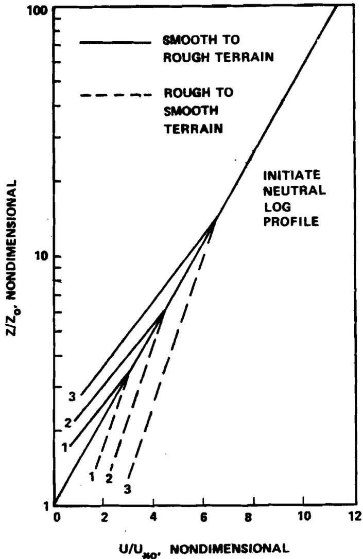
FIGURE 4. SCHEMATIC DIAGRAM OF THE VARIATION IN THE LOGARITHMIC WIND PROFILE DUE TO A DISCONTINUITY IN SURFACE ROUGHNESS. THE NUMBERS DENOTE THE SEQUENCE OF EVENTS FOLLOWING THE MEAN FLOW DOWNSTREAM FROM THE SURFACE ROUGHNESS DISCONTINUITY.  $u_{*0}$  AND  $z_0$  DENOTE THE UPSTREAM SURFACE FRICTION VELOCITY AND ROUGHNESS.
