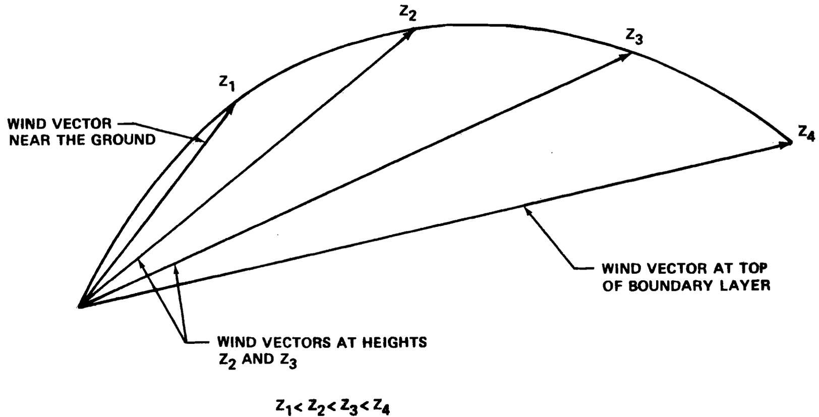
FIGURE 2. SCHEMATIC DIAGRAM OF HODOGRAPH OF ATMOSPHERIC BOUNDARY LAYER FLOW. NOTE THE CLOCKWISE TURNING OF THE WIND VECTOR AS ALTITUDE  $z$  INCREASES.
