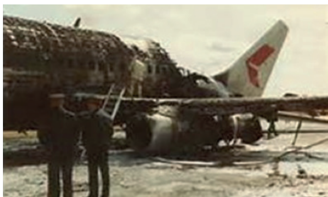
Wreckage of the B737-200 after an uncontained engine failure and fire during take-off at Calgary in March 1984.
