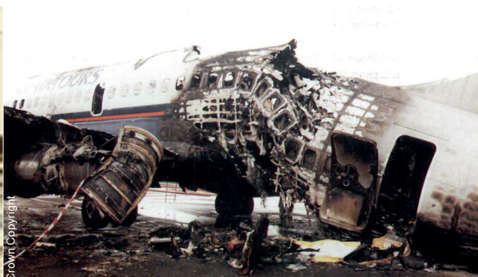
Wreckage of the B737-200 after an uncontained engine failure and fire during take-off at Manchester in August 1985.
