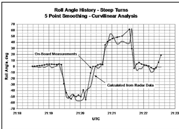
Figure 2. Calculated and measured bank angle during steep turns.
