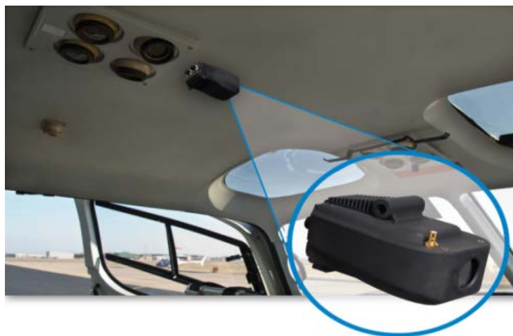
Fig 1: Vision 1000 system and mounting on cockpit ceiling on an AS350
