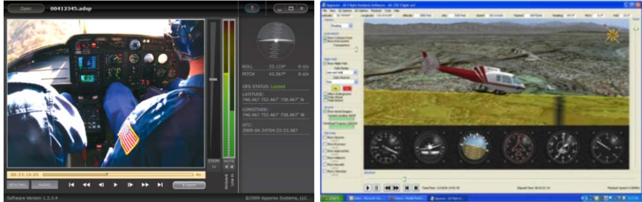
Fig. 2: Typical replay scene and 3D flightpath/attitude depiction, including instrument view
