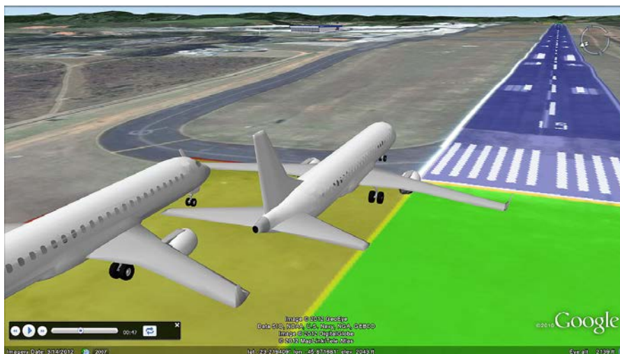
Figure 8. Simultaneous animation allows studying events involving more than one aircraft, as well as comparing two distinct landings of the same aircraft at the same airport, for instance. A runway may be drawn to improve visualization (especially interesting when a poor image is available from the geographic browser).
