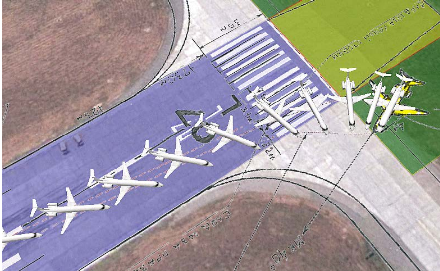
Figure 1. Runway overrun, shown “frame-by-frame”. A sketch made by the operator with tire tracks was placed over the terrain to rebuild the aircraft path and specially its heading during the final portion.
