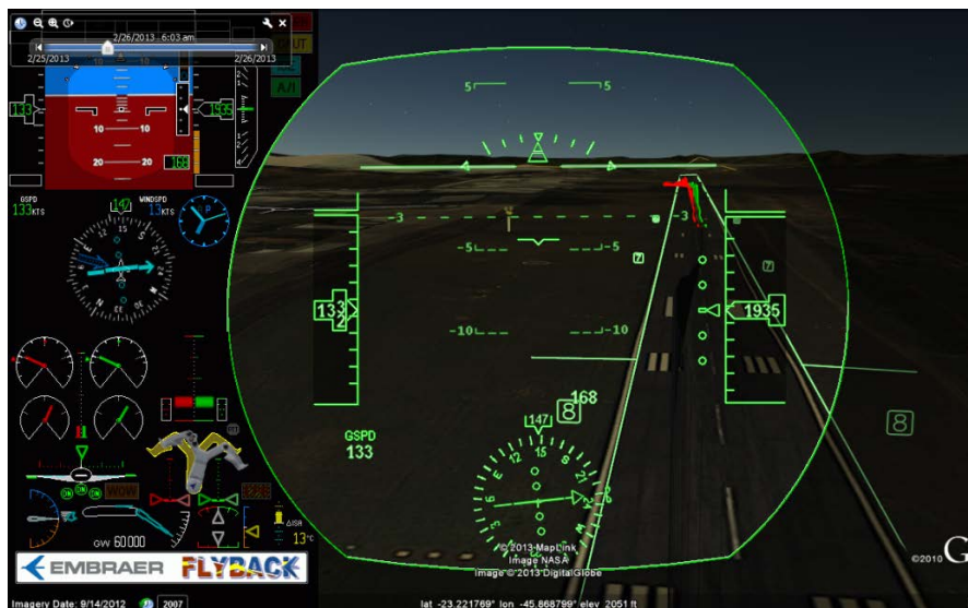
Figure 14. Event can be reviewed by the crew in a way they are familiar with. In this case, an animation of the HUD (Head-Up Display) running together with the "dashboard".
