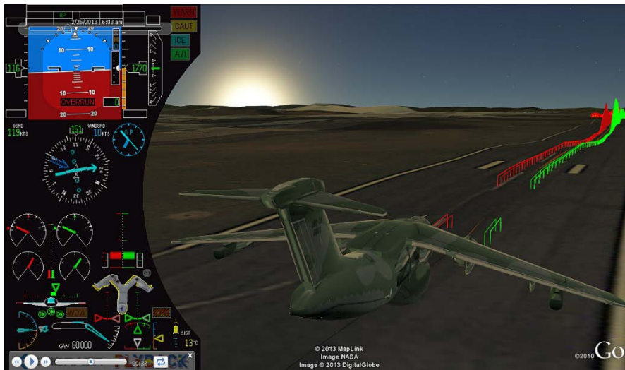
Figure 5. Bounced landing. Dashboard at left shows the main parameters (live). Curves represent brake pressure (only plotted if "Weight On Wheels" reading is true). The sun position is emphasized.
