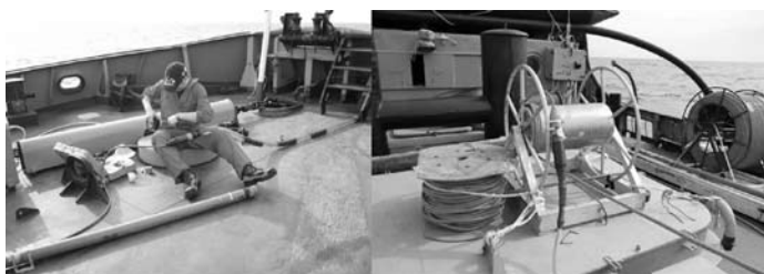
The participants preparing the tow fish and the cables for deployment.
