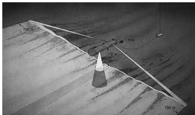
Figure 3. Towed side scan sonar towed at 70 m above the seabed and having a swath of 1,500 m.
