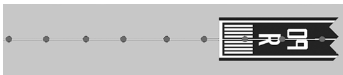
Figure 3. Sequence of geographical coordinates (in gray dots) defining the prolonged centerline calculated from a point on the runway. This sequence can then be used to calculate the SRTM terrain profile.
