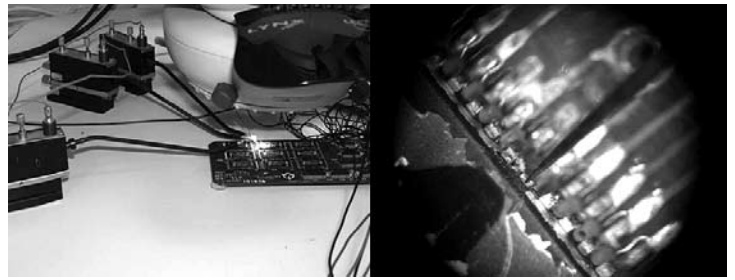
Figure 5. Readout of corroded memory chips from a flight recorder.
