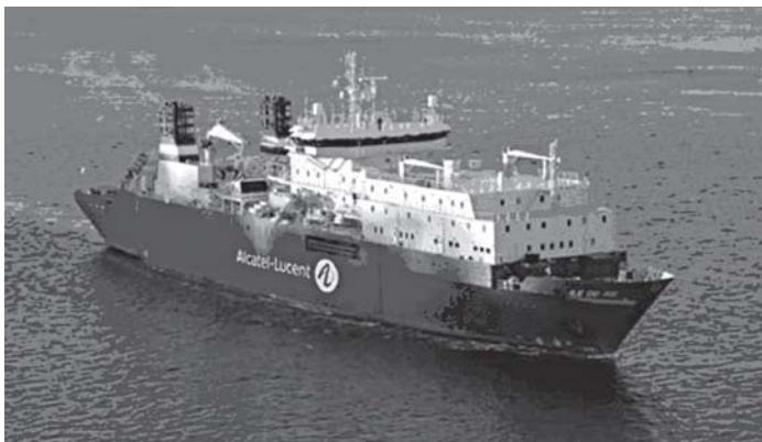
Figure 1. The Ile de Ré , a 140-meter-long cable-laying ship.
