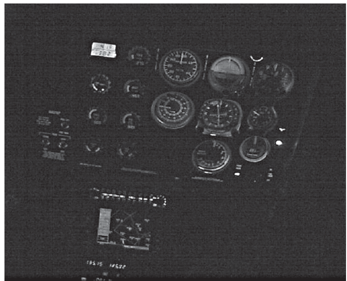
Figure 10. CIR image under low-light cockpit during NVG flight.
