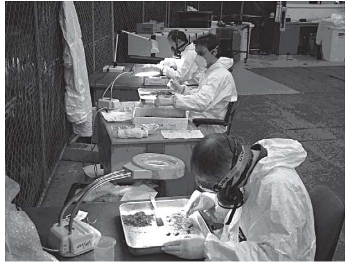
Figure 22. DSTO investigators carefully sifting through the sieved wreckage at DSTO Melbourne.
