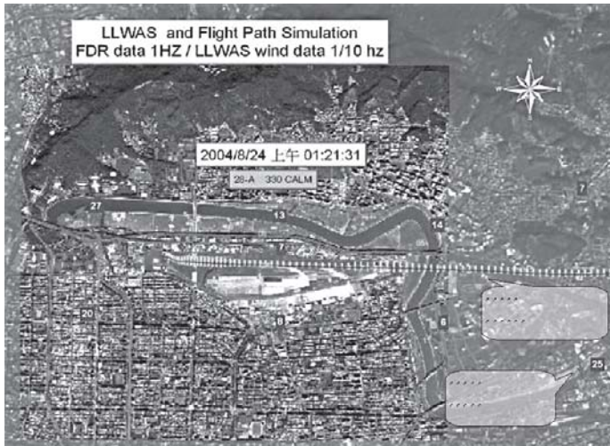
Figure 3. Superposition of LLWAS data and flightpath (an MD-82 encountered severe windshear at 120 ft AGL).
