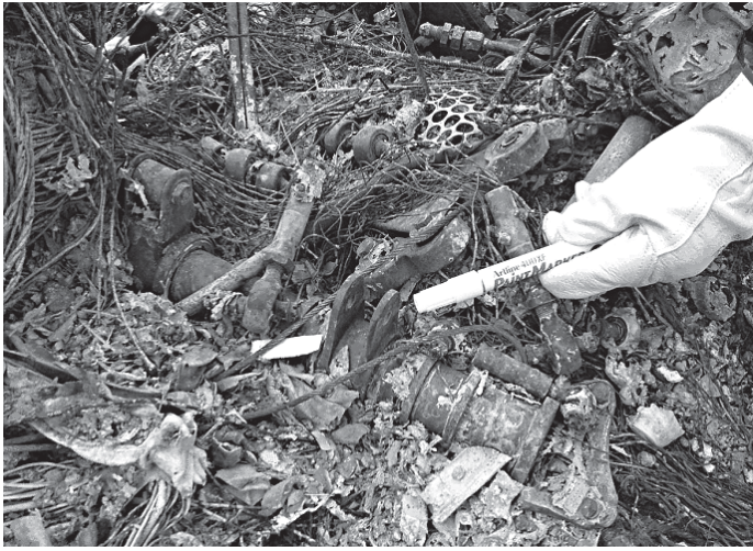
Figure 16. Location of the mixing unit, showing the lugs for the attachment of the fore/aft bellcrank.
