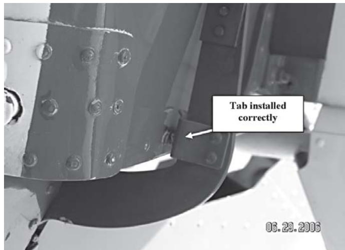
Figure 5: Exemplar Cessna 152 rudder stop installation—view of left stop plate against its stop bolt, i.e., full right rudder deflection.
