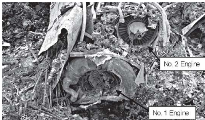
Figure 11. Photograph of the port (No. 1) and starboard engines.
