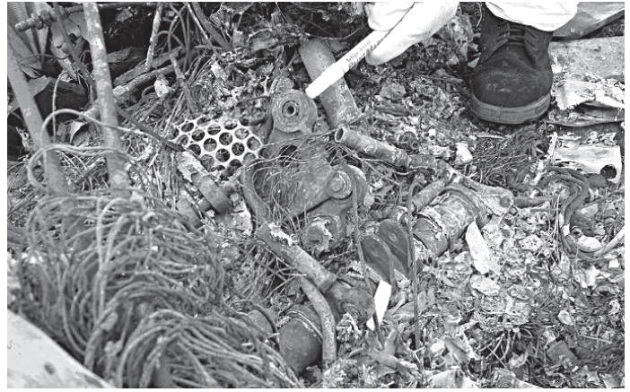
Figure 17. Location of the fore/aft bellcrank near the mixing unit.
