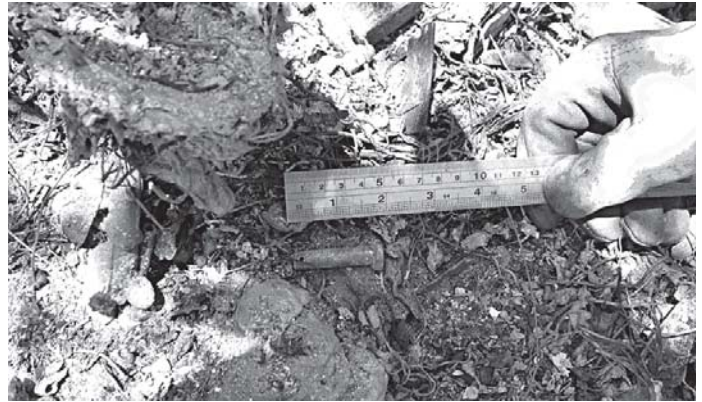
Figure 18. Area of location of the fore/aft bellcrank attachment bolt, discovered under debris.
