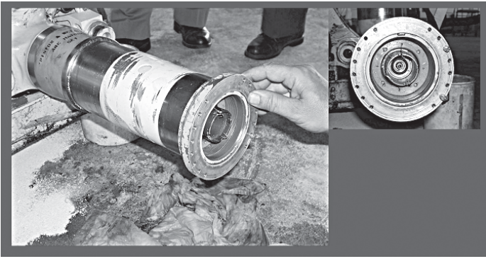
Photo 5. Detail of axle, spacer, and adapter (internal side).
