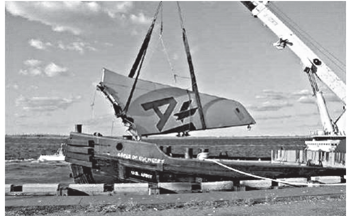
Figure 13. A300-600 composite vertical stabilizer that failed during American Airlines Flight 587 in November 2001 (NTSB 2004).
