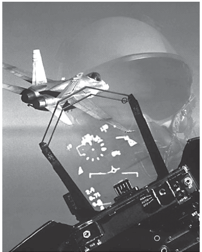
Photo 1. HUD display from the cockpit of the F/A-18 Hornet.
