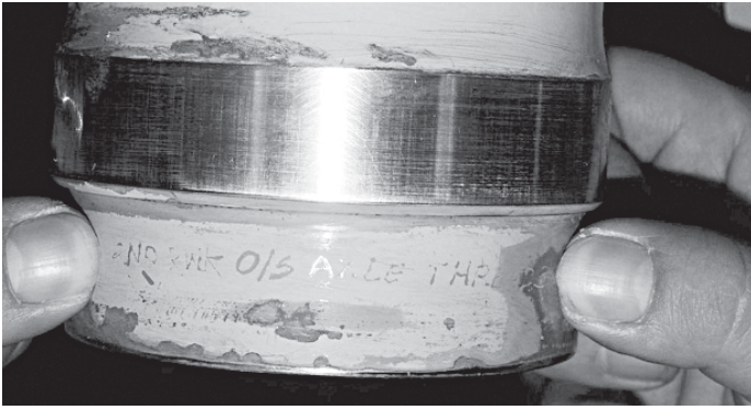
Photo 9. Axle tip vibro engraved inscription, covered by painting (view after painting removal).
