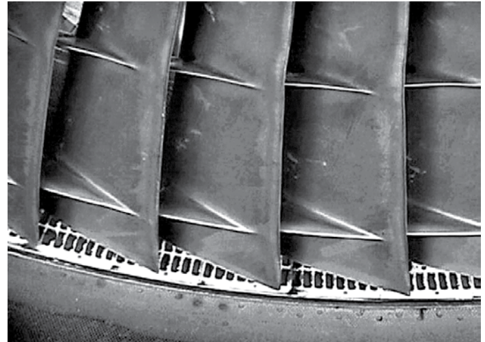
Figure 7. Fan blade tips seized into fan case.
