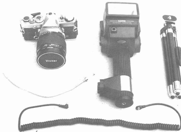
Photo No. 1. Minimum equipment. Camera, lens, electronic flash, tripod, cable release and flash extension cord.
