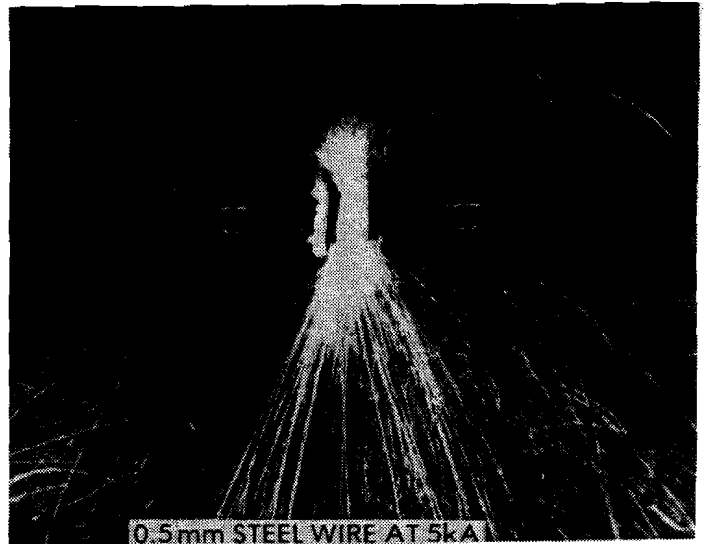
Figure 7 Resistive heating and explosive vaporization of conductors. (USAF photo)
