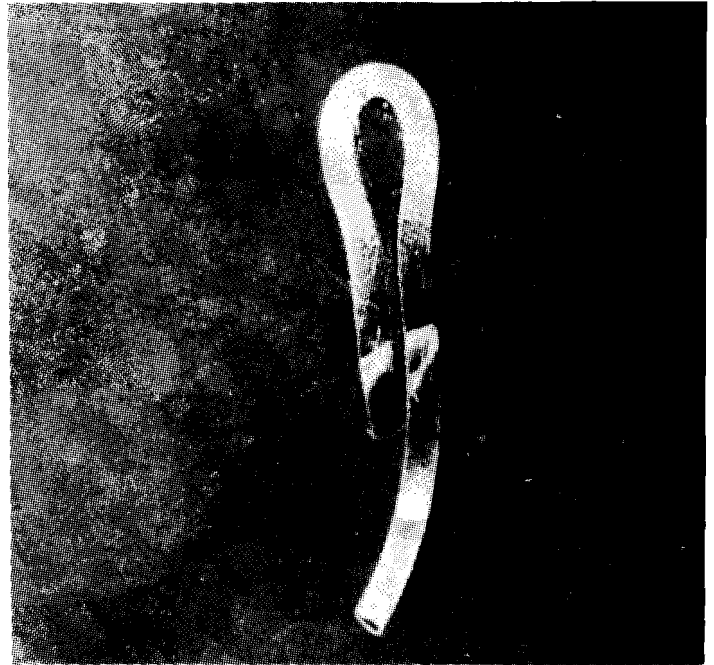
Figure 1 - Section of buckled exhaust pipe which has been mounted and polished in readiness for hardness measurements.
