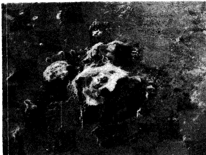
Figure 13a SEM Micrograph of "Burning Bronze" Pit
