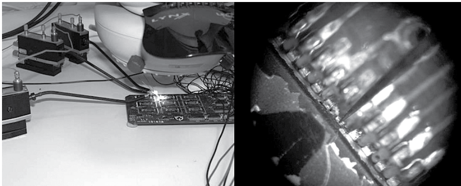
Figure 5. Readout of corroded memory chips from a flight recorder.
