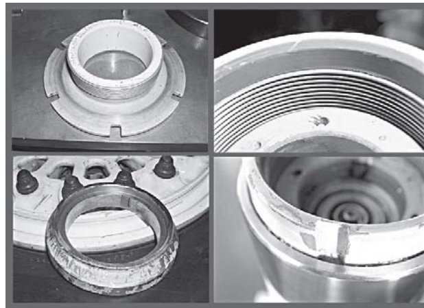
Photo 5. Detail of axle, spacer, and adapter (internal side), above. Photo 6. Detail of axle thread, nut, and anti-rotating devices (no damage), left.
