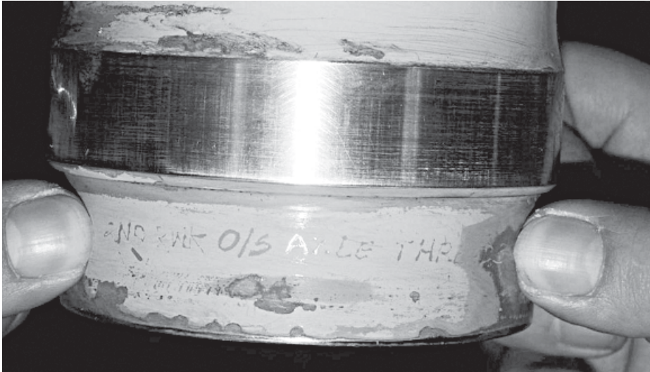
Photo 9. Axle tip vibro engraved inscription, covered by painting (view after painting removal).
