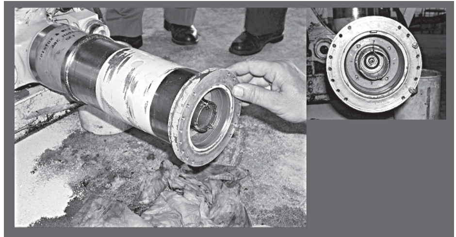
Photo 5. Detail of axle, spacer, and adapter (internal side), above. Photo 6. Detail of axle thread, nut, and anti-rotating devices (no damage), left.
