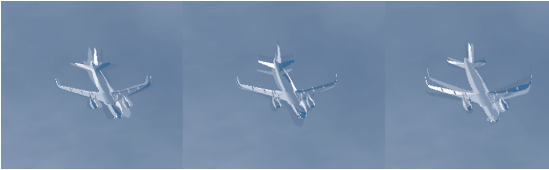
Figure 9. Attitude error +/-10 degrees visualized (blue/cyan), heading (left), pitch (middle), roll (right).
