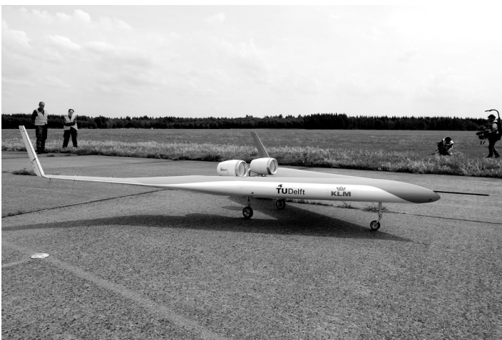
A scale model of the Flying-V on the runway during flight testing.
