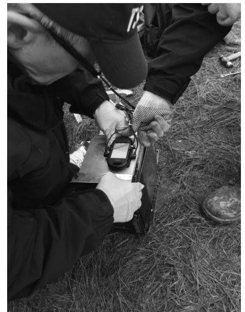
Although not required by regulation, a cell phone that had GPS, voice recording, and accelerometer capabilities was attached to the Mitsubishi aircraft's radio.
