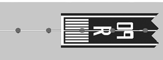
Figure 3. Sequence of geographical coordinates (gray dots) defining the prolonged centerline calculated from a point on the runway. This sequence can then be used to calculate the SRTM terrain profile.
