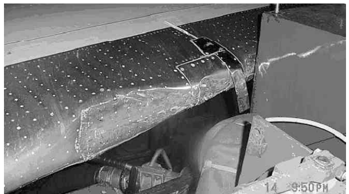
Figure 1 (top): Leading edge slats 4 and 5 damaged.
